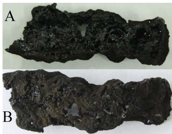
Figure 6. Photographs of the inner (A) and outer (B) carbon residues at the bottom of TPIU211 when the burning is up to 60 s. [Color figure can be viewed in the online issue, which is available at wileyonlinelibrary.com .]
